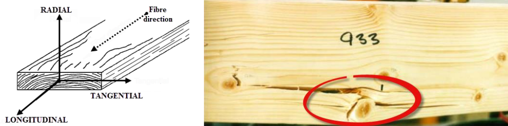
Figure 2: Left: Grain directions of wood members; Right: visual failure around local defects of loaded timber elements, both taken from [10]
