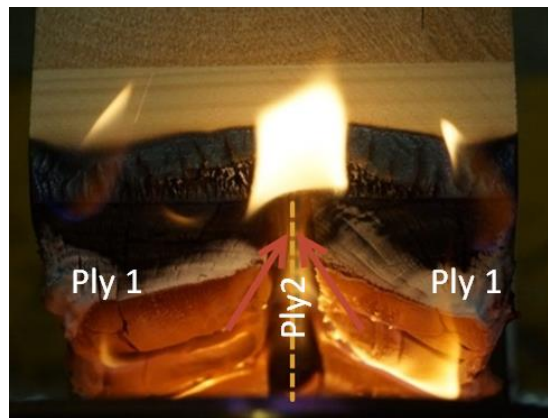
Figure 36: Significantly increased charring along bond line (Test type M)
