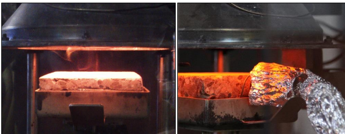
Figure 12. Two samples being heated under the cone at 85 \text{ kW/m}^2 : the left picture shows an experiment for measurement of mass only (note the cloud of water vapor which is visible at the top of the sample); the right picture shows the counterpart experiment with thermocouples connected for recording the temperatures.
