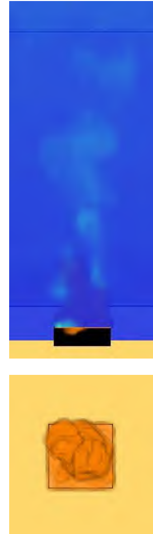
A simulation of oscillatory combustion by a heptane pool fire in an enclosure (side view and top view).
