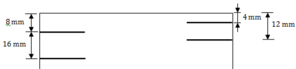
Figure 14 – Schematic of the thermocouple position in the sample.
