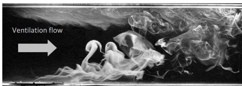
Figure 2.4 Photograph of a small scale tunnel fire during the occurrence of back-layering. Taken from Colella [24] who has adapted it from Wu and Bakar [20].
