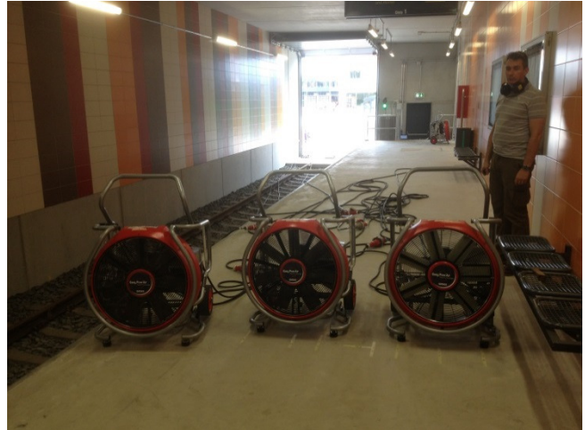
Figure 4.13 Three fans placed on the platform in the Frankfurt subway building. The fans are positioned with reference to the middle line of the stairs. From right to left: -25cm, +67cm and +150cm. The stairs are behind the photographer. The fan which is right in the picture is addressed as 'left' in the text and vice versa.
