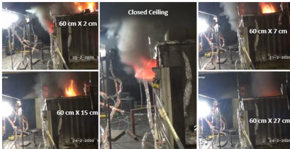
Figure 12: Screenshots for the external flaming for the central opening tests (during the steady state)
