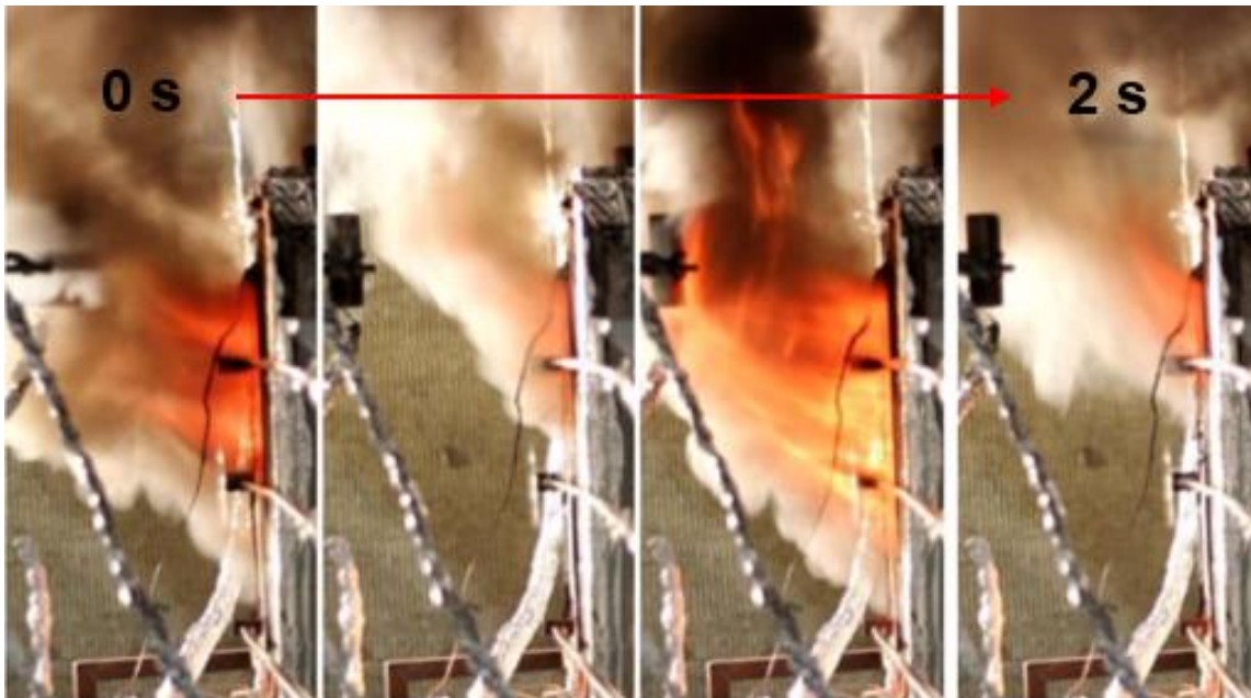
Figure 19: Oscillating Flames in the 0.05x0.05 m corner opening case
