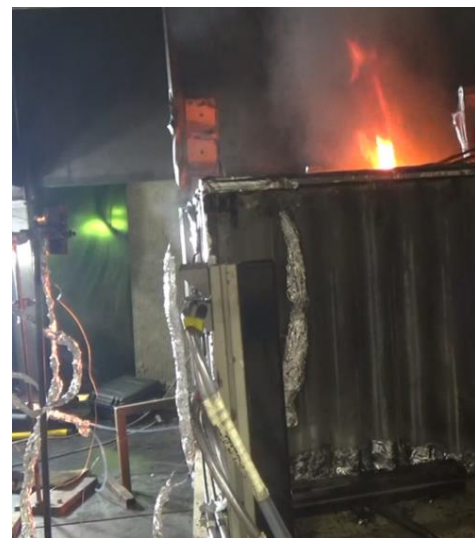
Figure 62: Validation of the external flaming for the 27_open_1 case
