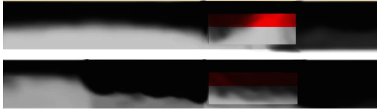
Figure 4.10: Comparison of FDS SMOKE3D file when placing water nozzles at different locations. Top: Directly above fire; bottom: 10 m Upstream of fire
