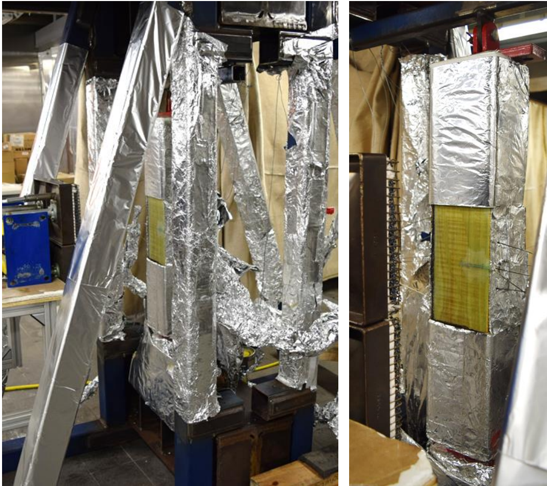
Figure 5. Loading frame designed by Chowdhury [49], with new pin-pin support.
