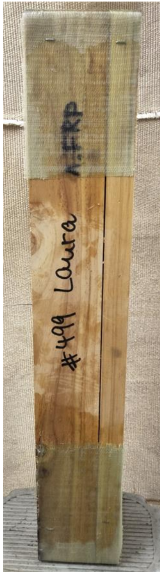
Figure 4. Cured 'CLT with FRP' samples without insulation (Top and bottom left and middle) and with insulation (Bottom right).
