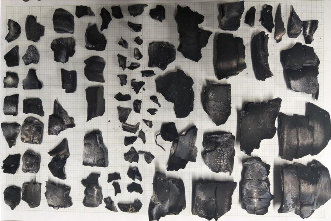
Figure 30. Fallen char from CLT without FRP at 50 kW/m 2 (5.CLT.P).
