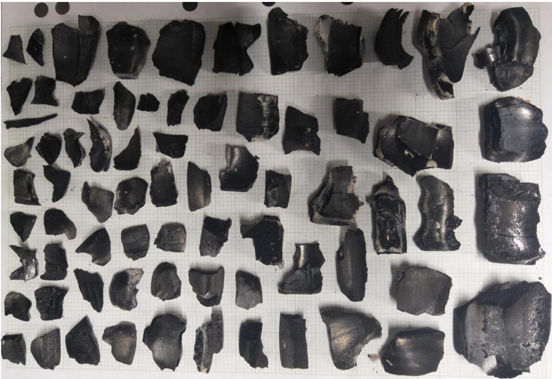
Figure 31. Fallen char from CLT without FRP at 50 kW/m 2 (6.CLT.P).
