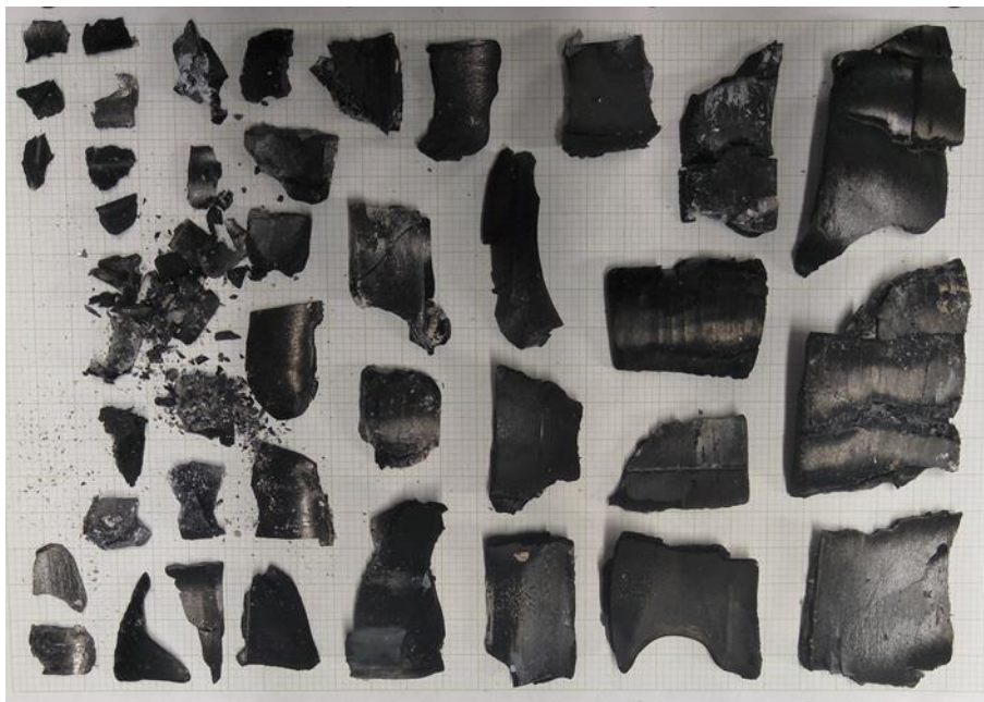
Figure 29. Fallen char from CLT without FRP at 20 kW/m 2 (2.CL.T.P).
