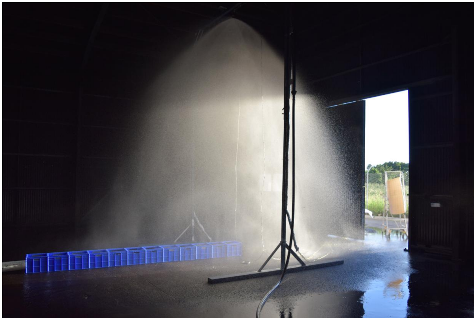
Figure 3.5: 'Pan test' to derive water distribution
