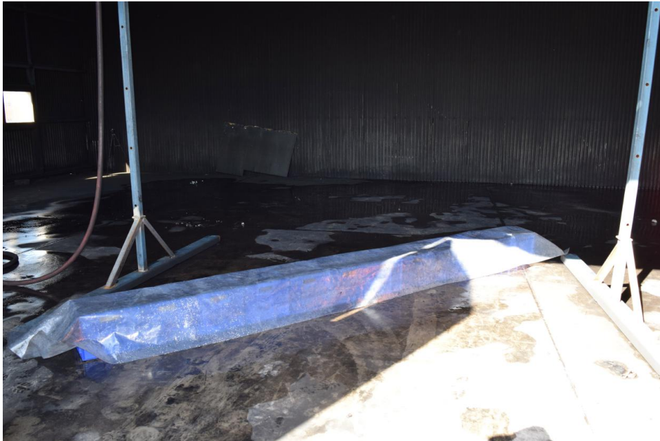
Figure 3.6: Diagonal 'Pan test' to assess radial symmetry
