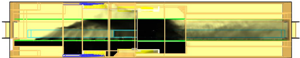
Figure 77 - Top View of smoke spread. 500 kW Fire. 420 Seconds. Side Exhaust, Revised PSD, Stairs Enclosed
