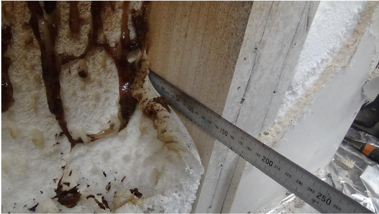
Figure 40: Measurement of EPS in the bottom part of the sample after the test
