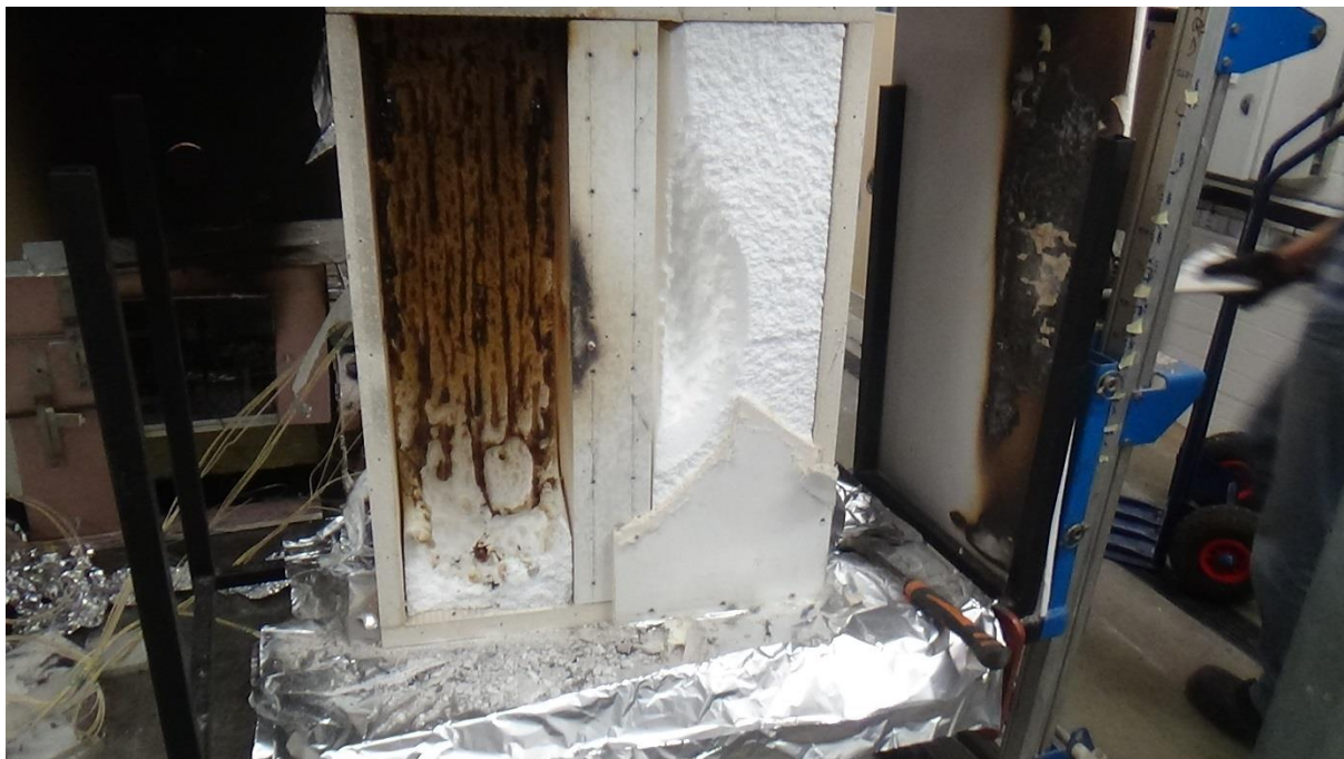
Figure 39: Inside of sample after the test
