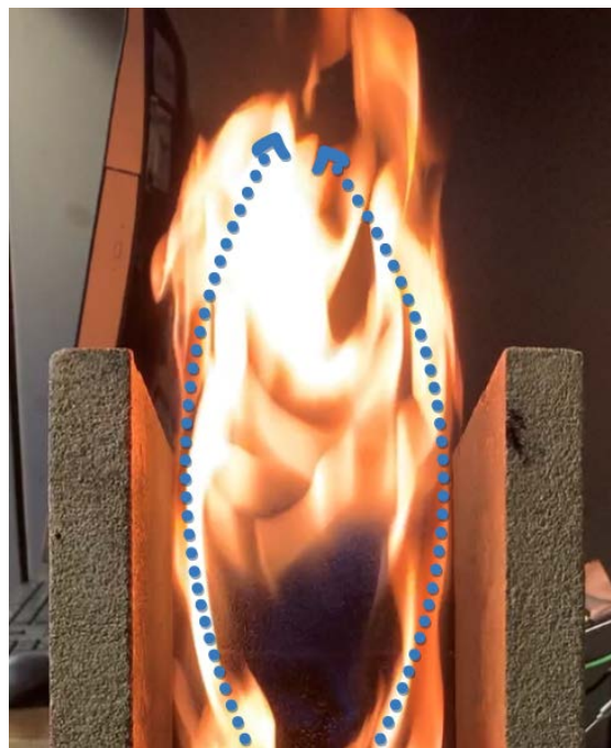
Figure 28. Flames curving towards the centreline at the top of the trench
