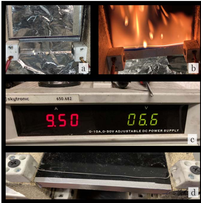
Figure 20. Ignition set up. (a) wire before the ignition (b) wire at the beginning of the test (c) power supply parameters (d) foil protection of the bottom part
