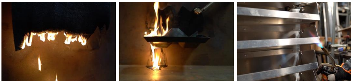
Figure 18. Reaction to Fire of Supportive Components (a) Synthetic & Natural Blend, (b) Polypropylene, & (c) Aluminum. Source: Green Living Technologies INTL [39]
