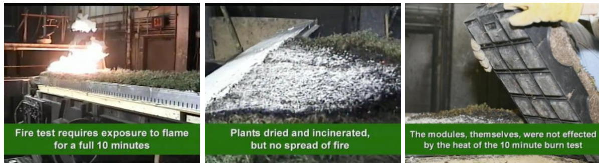
Figure 14. Fire Test on Green Roof (a) Flame exposure on vegetation, (b) Inspection of growing medium, (c) Inspection of modules Source: LifeRoof Global LLC [38]
