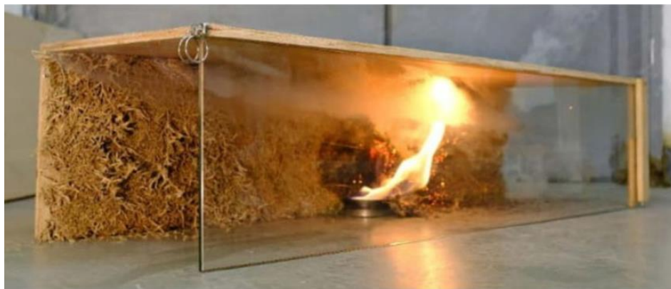
Figure 21. Scale Model of a Green Corridor Fire at 140 seconds Source: Study on the fire growth in underground green corridors [37]
