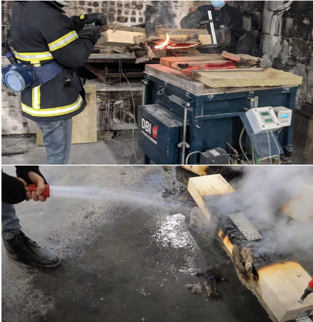
Figure 22. Removal of test sample 1 from the oven (top), extinguishment of sample 2 (bottom)
