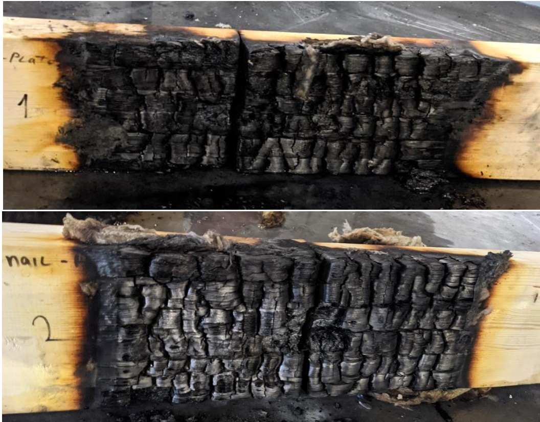
Figure 27. Exposed side of the Test 1 and 2 after 30 minutes of the ISO 834 fire curve
