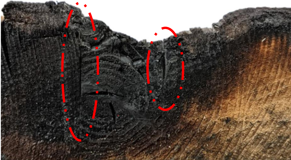
Figure 31. First cut of the second test showing signs of delamination
