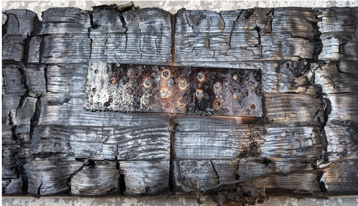
Figure 28. Exposed side of the protected sample after 30 minutes of the ISO 834 fire curve (test 4)
