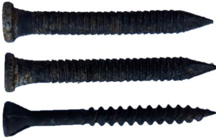
Figure 34. Fasteners after being exposed to the ISO 834 curve, from test 1, 2 and 3 (from top to bottom)
