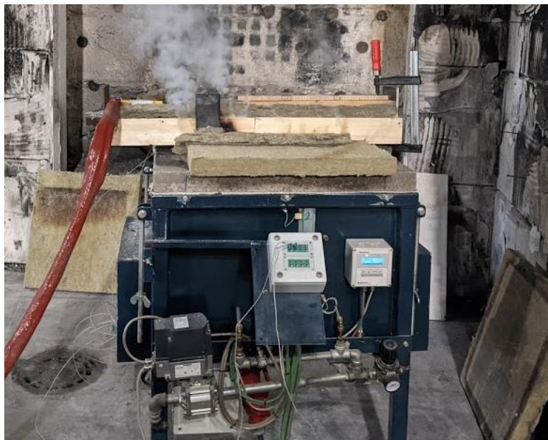
Figure 21. Specimen 1 exposed to the fire curve
