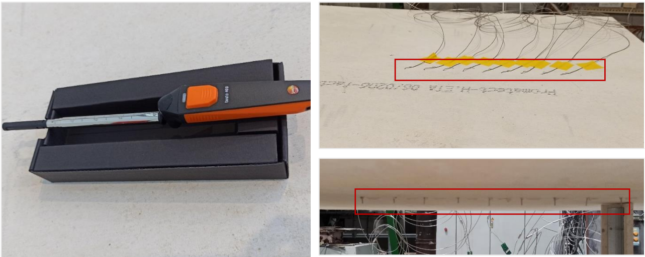
Figure 14: Thermal anemometer (Left) and thermocouples (Right) for flowrate and temperature measurement
