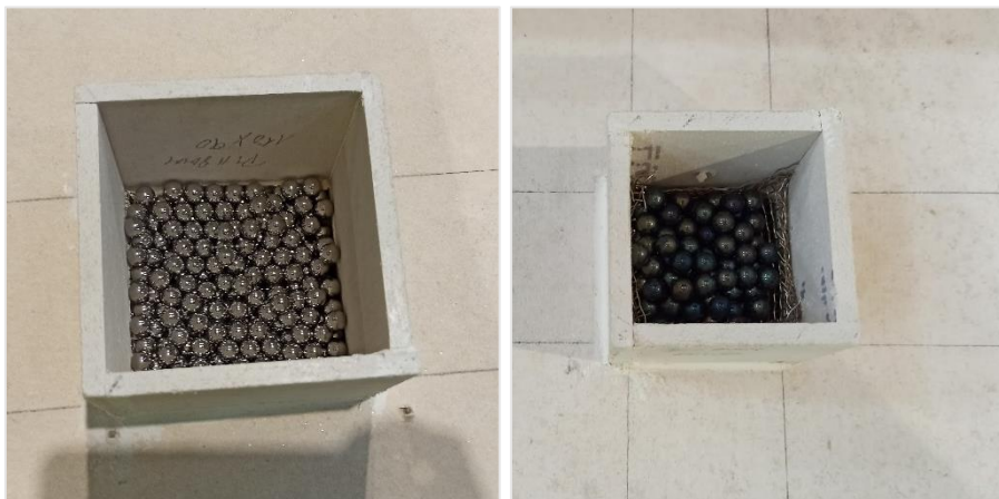
Figure 11: Steel mesh and balls to homogenize the hot air flow (E5)
