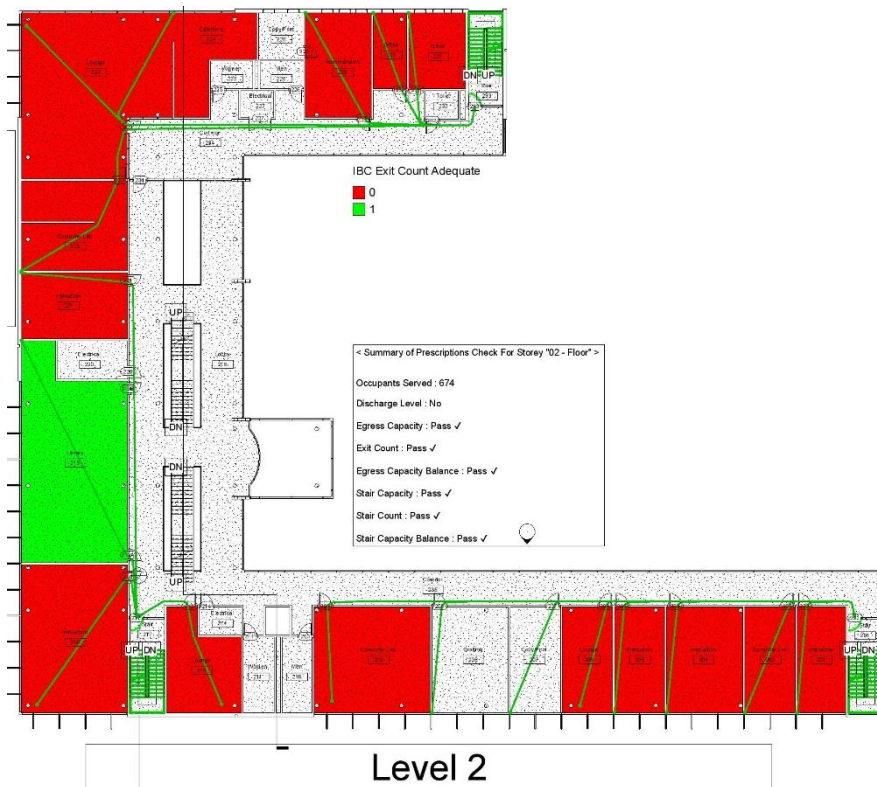
Figure 29 – Prescription review results (case study 1) Rooms are colored based on the outcome: Green: Pass – Red: Fail
