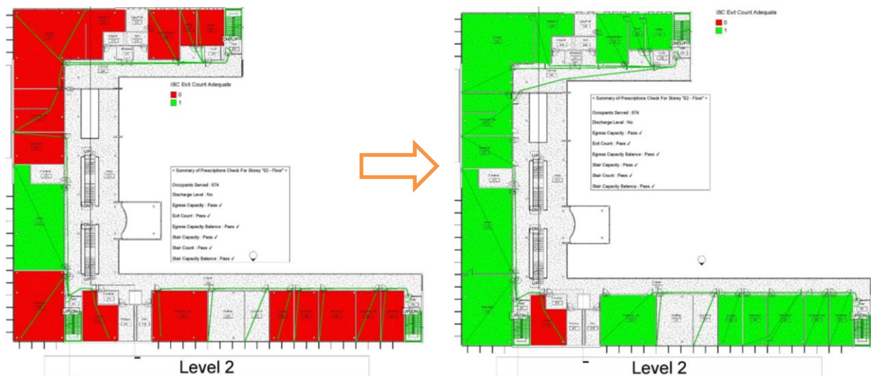
Figure 30 – Exit count check prior and after modification of the model (case study 1)
