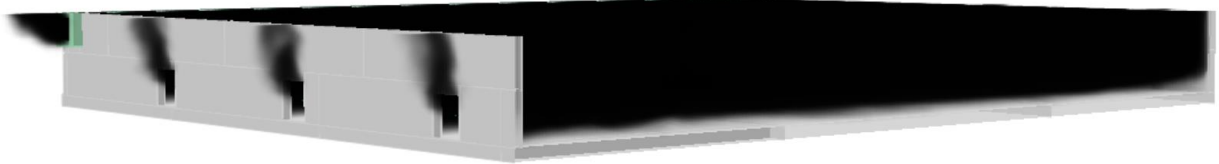
Figure 23: 3D Smoke visualization showing the smoke flow from the SED outlet (top left, green box) and the smoke layer deepening to almost floor level in the compartment and smoke flows out from the air inlet openings.
