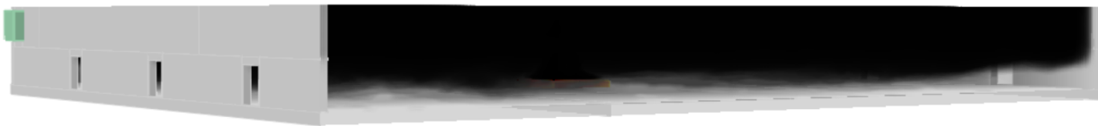
Figure 27: 3D Smoke visualization showing a higher smoke layer in the compartment and no smoke outflow from the air inlet openings.
