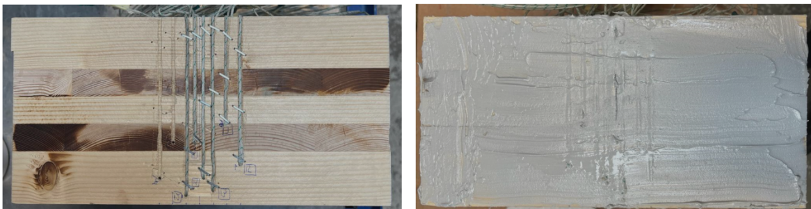
Figure 3.9: Installation of second group thermocouples (left), and application of fireproof cement
