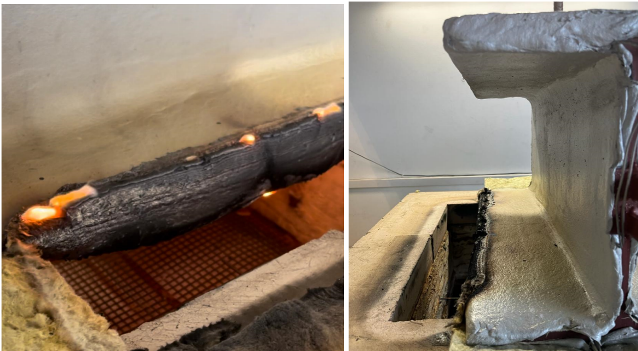
((a)) Combustion on the intumescent coating
