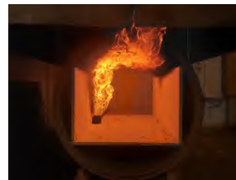
Figure 5.23: Propane Tunnel Side - 0.75L/s
