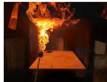
Figure 5.15: Propane Flat Side - 0.75L/s
