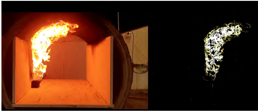
Figure 5.24: Result of the video analysis performed on the experiment's video recordings.
