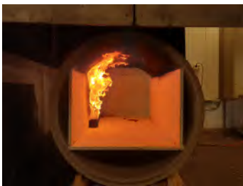
Figure 5.19: Propane Tunnel Side - 0.3L/s
