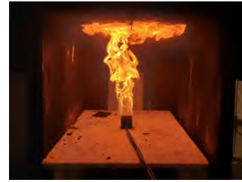
Figure 5.10: Propane Flat Centre - 0.5L/s
