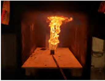
Figure 5.8: Propane Flat Centre - 0.3L/s
