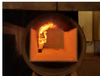
Figure 5.20: Propane Tunnel side - 0.4L/s
