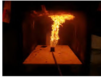
Figure 5.9: Propane Flat Centre - 0.4L/s
