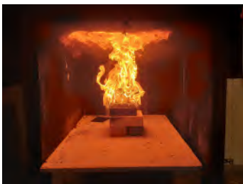
Figure 5.5: Heptane Flat Centre Elevated
