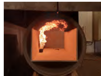
Figure 5.21: Propane Tunnel Side - 0.5L/s
