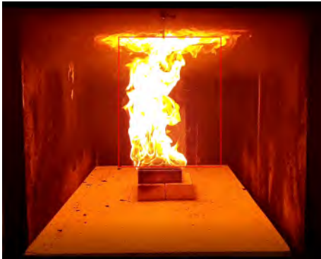
Figure 5.25: Results from the bounding rectangle for heptane in the flat ceiling setup.
