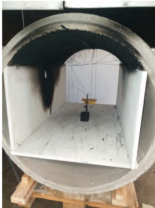
Figure 4.2: Curved ceiling setup
