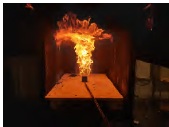
Figure 5.14: Propane Flat Centre - 0.75L/s
