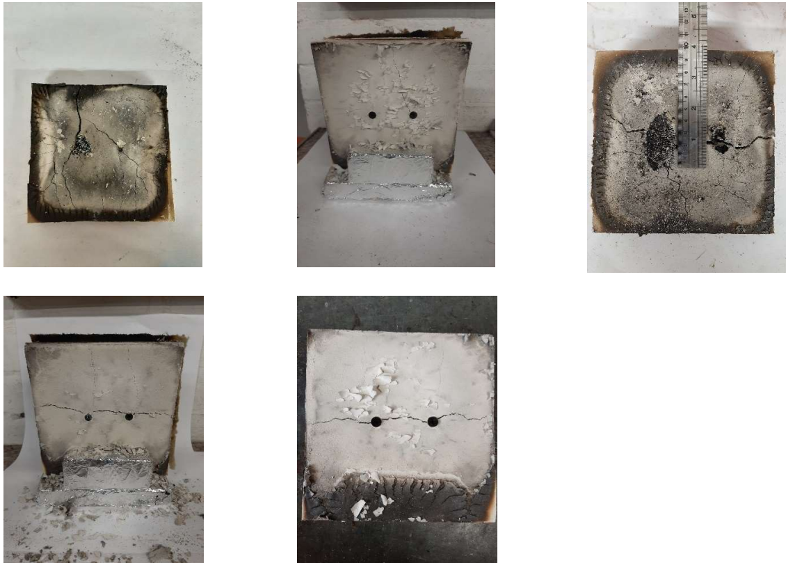
Figure 13: Thermal degradation of plasterboard observed for experiments
