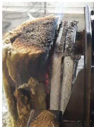
Figure 11: Experiment 5b falling forward, leading to minor section of exposed timber
