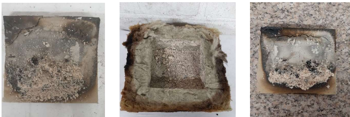
(a) Char remains on screw after experiment 4a and ash (b) Ash remains within insulation pocket after experiment 5a: (c) Char remains on screw after experiment 5b
